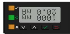
Figure 32. LE550 Inverted Display Orientation
