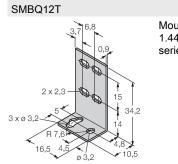
3073722 Mounting bracket; material VA 1.4401, for photoelectric sensor, Q12 series
