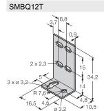
Mounting bracket; material VA 1.4401, for photoelectric sensor, Q12 series
