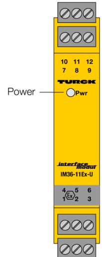
The 1-channel potentiometer amplifier IM36-11EX-U/24VDC is designed to transmit signals from 3 or 5-wire potentiometers galvanically isolated from the Ex area to the non-Ex area and to convert them into normalized 0...10 V analog signals. The resistance value of the wiper contact, ranging from 0 Ω to the nominal resistance value (final value) of the potentiometer, is detected and linearly processed.
