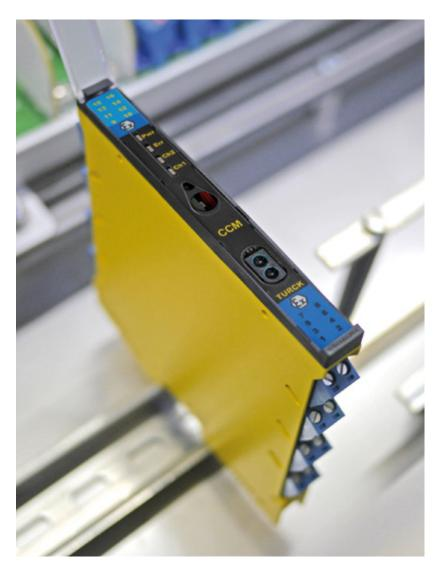
The IMX12-CCM launched a year ago is primarily designed for use in the Ex area thanks to its intrinsically safe 2-wire isolating transducer interfaces
