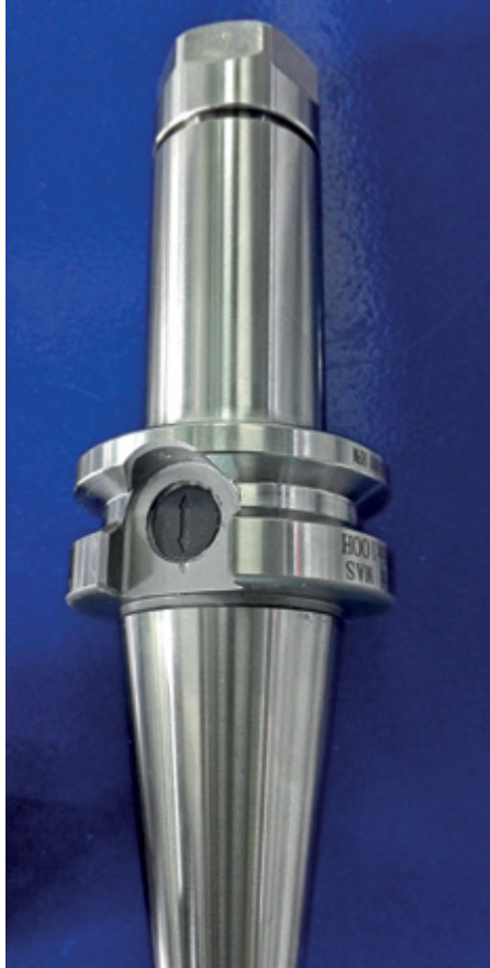
Cutting tool holder with embedded RFID tag
