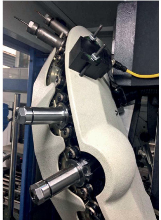
The RFID read/write head is fitted to the back of the tool turret and reliably detects the tag in the tool holder thanks to its extended range through the paneling
